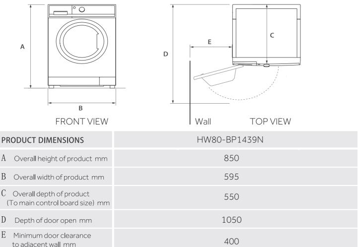
Note: The exact height of your washer is dependent on how far the feet are extended from the base of the machine. The space where you install your washer needs to be at least 40mm wider and 20mm deeper than its dimensions.
